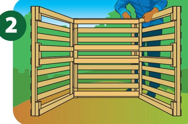
Screw three of the pallets together. Attach bolt latches to the front edge and last pallet to make a removable door
